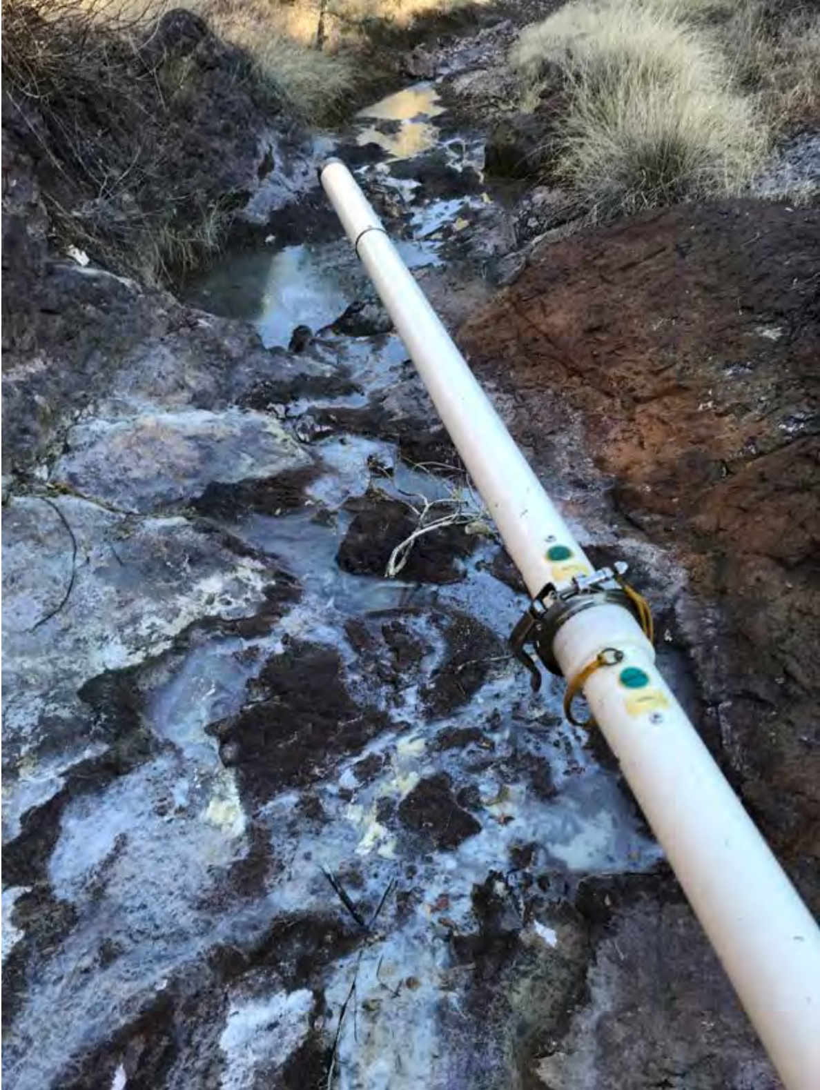
Figure 5.4. EM-31 device with booms attached over areas downstream from the adit where the white precipitate was found. These areas were harder to get accurate distance readings due to difficult terrain and the size of the EM-31 device.
