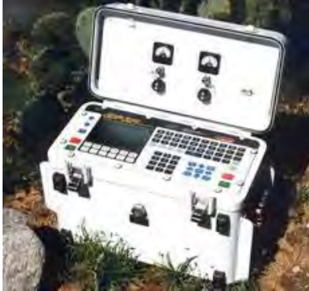
Figure 3.1b. Geophysical Data Receiver-32 II: instrument used in collection of data.
